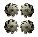
With the help of mecanum wheels, robot kit can move to all direction. Moving all four wheels in the same direction causes forward/backward movement, running left/right sides in opposite directions causes rotation, and running front and rear in opposite directions causes sideways movement.
