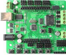
Arduino 328 is a microcontroller board. The USB port can be used for download of own programs and for transmitting data to the PC.
